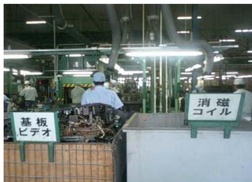
Fig. 7 Takeoff of Boards and Coils
